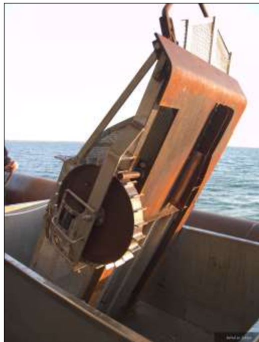
Foto 4: bodem schaar nog half in de kist. Photo 4: bottom dredge still half in storage box
