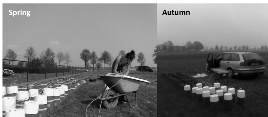
Figure 1.6. Taking gas flux measurements from intact soil columns under field conditions in two different seasons.
