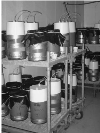
Figure 1.5. Mesocosms ready for N_2O and CO_2 fluxes under controlled laboratory conditions.
