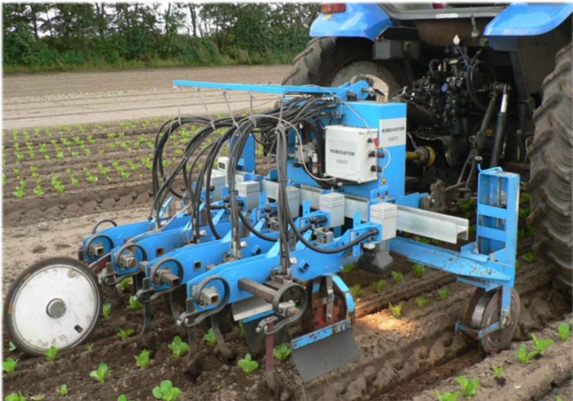
Figuur 9. Robovator, fa Poulsen, in-de-rij schoffelmachine.
