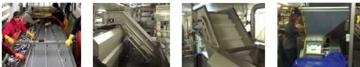
Figure 3.4 Discard handling on board of the Carolien (SCH81). From left to right: discard path on the sorting conveyor, conveyor belt for discards into the discard hold, conveyor belt out of the discard hold and the mincing device.
