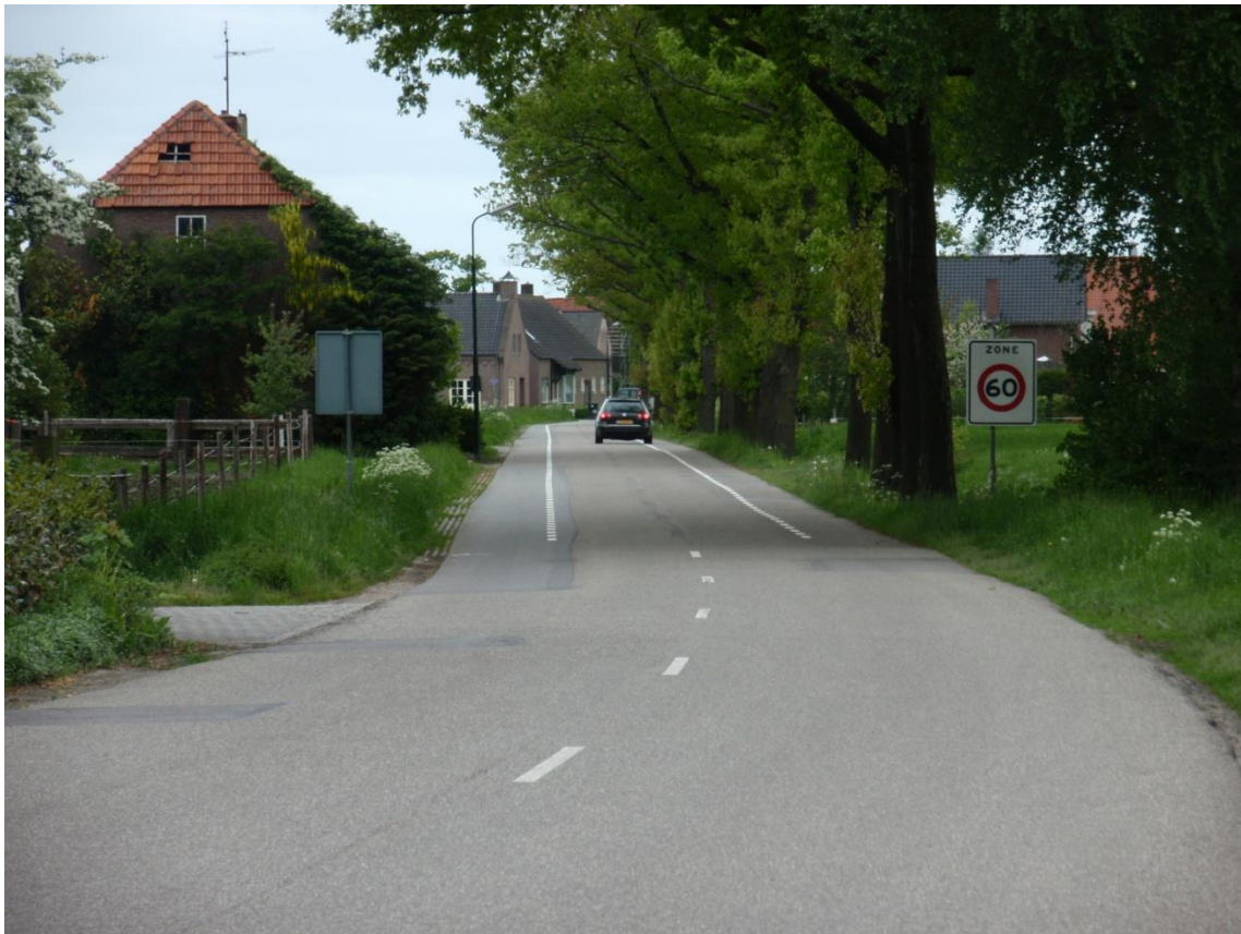
Figure 10: The municipality border on the local connection Alphen - Baarle - Nassau via Terover. The speed limit and the signalling changes, but the road width does not change.
