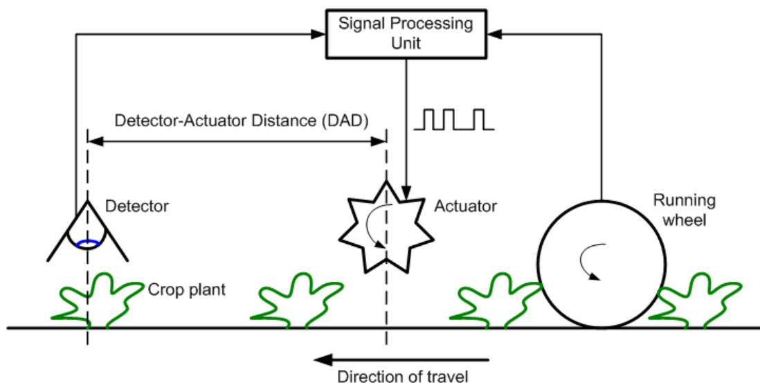
Figure 1. Schematic lay-out of a machine for intra-row weed control defining the Detector-Actuator Distance (DAD).
