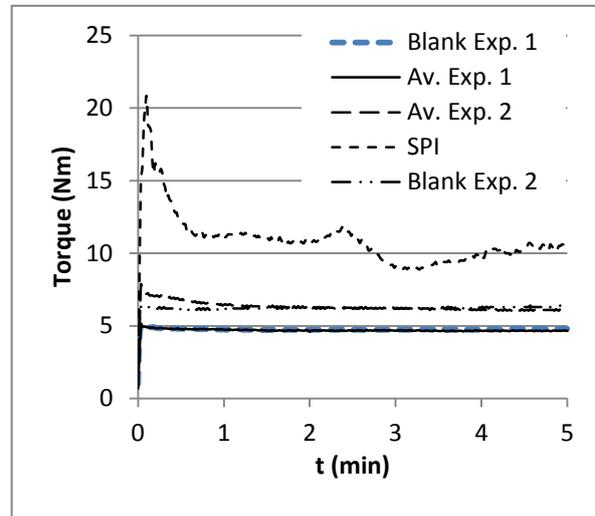
Figure 1. Comparison of the torque profile of soy protein isolate (SPI) and the average profiles obtained from the treatments and the blanks in Experiment 1 and Experiment 2.
