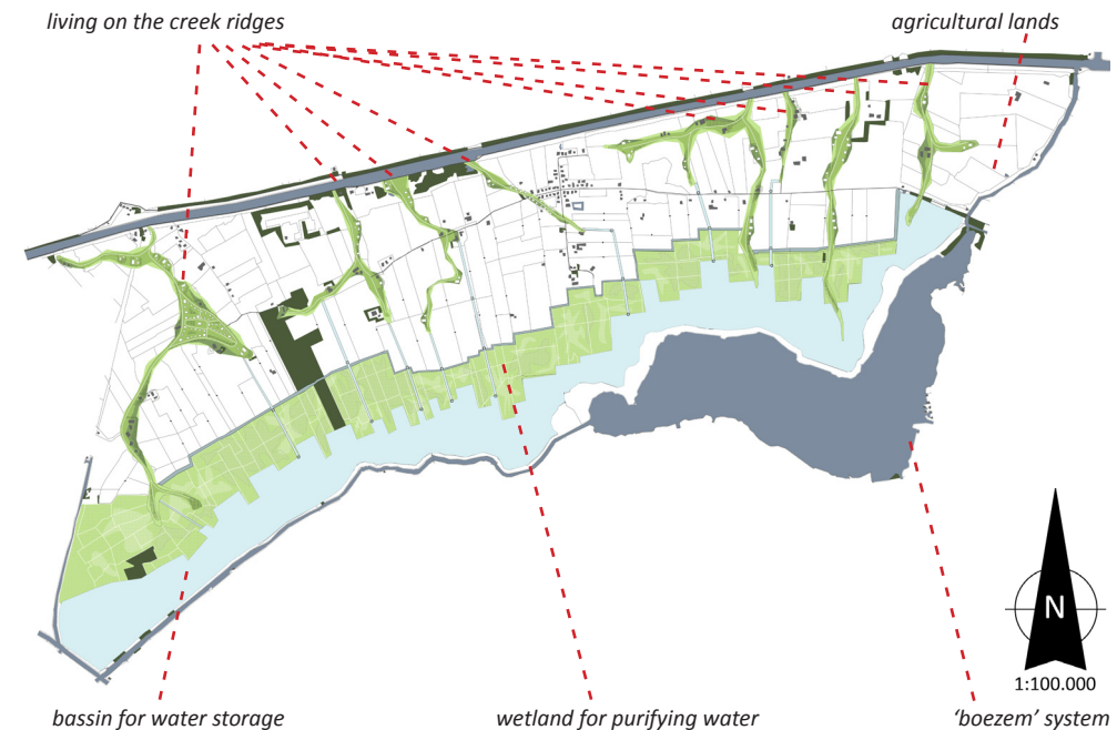
figure 58; 'the wetlands archipelago'; living on the higher grounds, storing and purifying water on the low grounds
