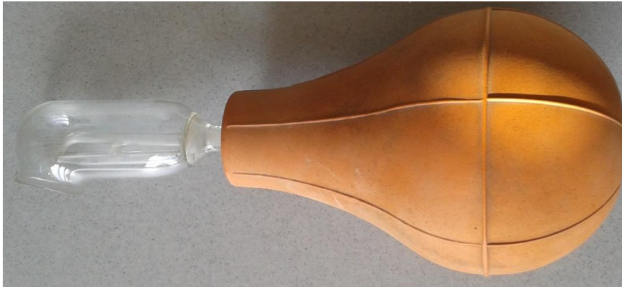
Figure 4: the hairdressers spray used to apply the spore suspension on the detached leaves.
