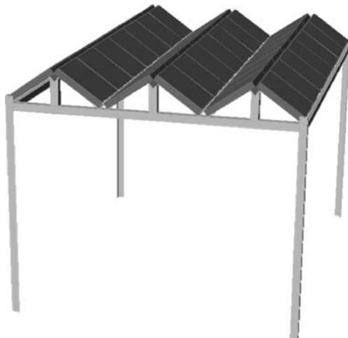
**Fig. 2** Platform that was placed at the study site containing 42 tiles, sponges were attached on every tile. Size platform: 2.5-m×1.6-m×1.2-m
