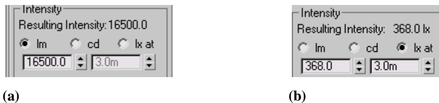
Fig. 20. (a) The first window shows resulting intensity from the luminaire in lumens (16500 lm), as in the research has been used. (b) The second shows the parameters election with regards to the Isolux diagram ( H=3 meters and E_{max}=368 luxes).
