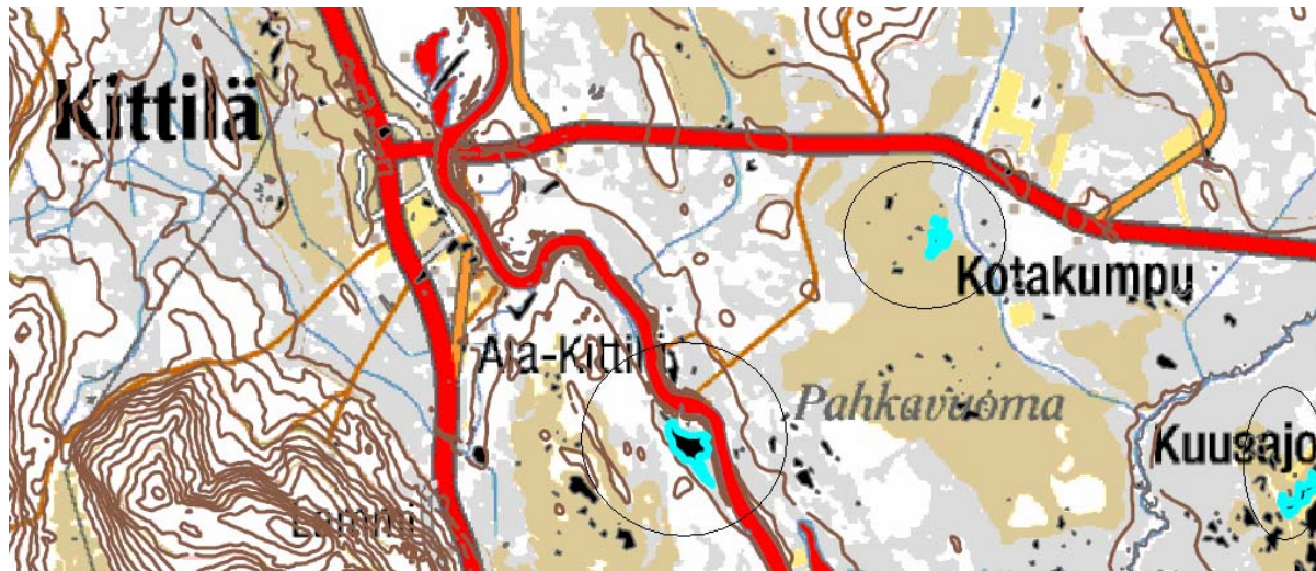
Figure 4 Potential flood detention basins detected (black spots) from the RADARSAT image acquired on 30.5.2005 during a flood in the city of Kittilä: without a field survey, the black areas within circles were defined as the most appropriate. Areas identified are outside of typically water-covered areas (red colour).
