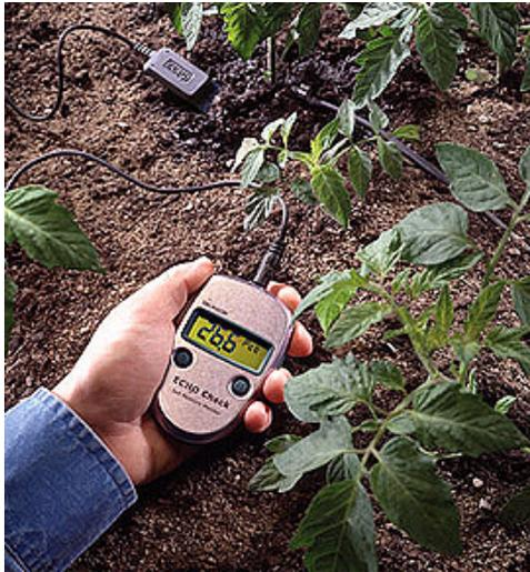
The ECH<sub>2</sub>O probes come pre-calibrated for most soil types, although specific calibrations for a particular soil are also possible. The standard calibration for the probe, which is suitable for soils with low to moderate sand content, is:
