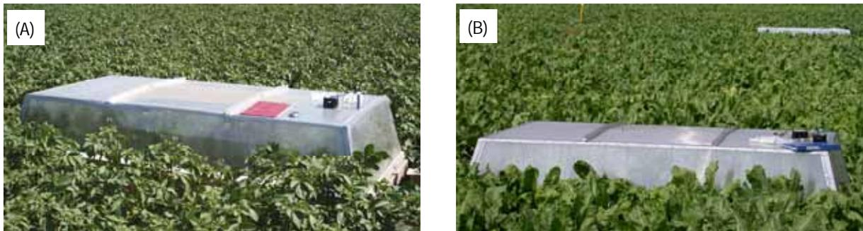
Flux chambers use de law of conservation of mass to determine the gas exchange between the soil surface and the atmosphere:
