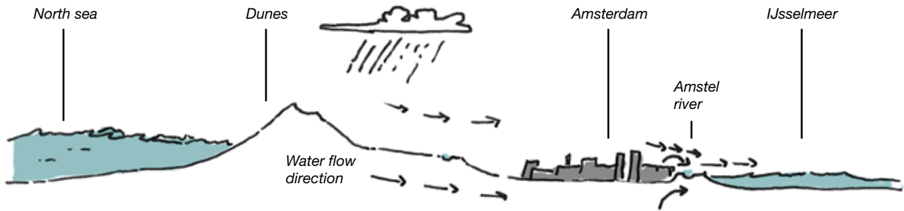
Image 8.3. Cross section of the Amsterdam area, showing the outflow of water from the polders, via the Amstel river towards the IJsselmeer.
