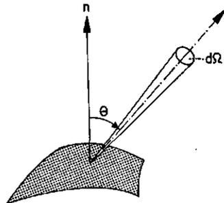
FIG. 1. Infinitesimal solid angle  $d\Omega$  including angle  $\theta$  with normal  $n$  at surface in radiating point.
