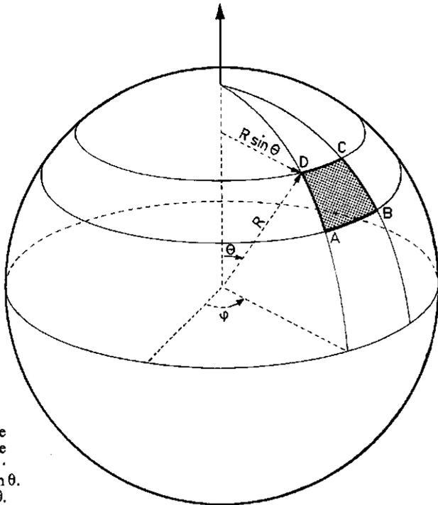
FIG. 3. Spherical coordinate system and surface element  $dS = AD \cdot DC = R d\theta \cdot R \sin \theta$ .
