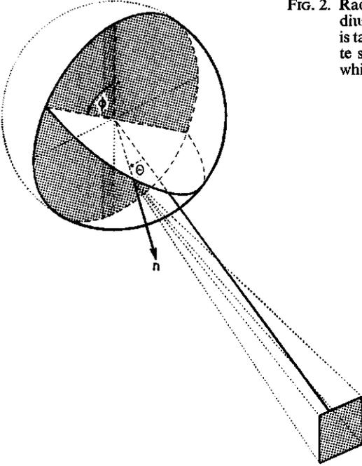
FIG. 2. Radiating hemisphere and receptor. Radiusvector from centre of sphere to receptor is taken as polar axis of spherical coordinate system. Receptor is parallel to plane in which azimuth  $\Phi$  is measured.
