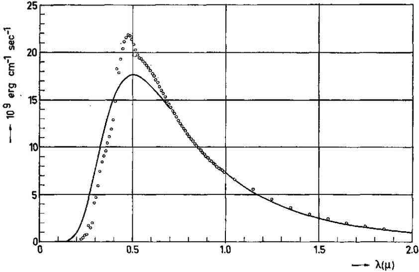
FIG. 4. Theoretical and empirical energy distribution. Full drawn curve presents theoretical value of  $E^+$ , experimental values are represented by dots.
