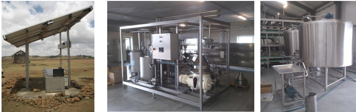
Figure 21: Solar panel milk cooler and a container size milk factory, produced in the Netherlands for a farmer cooperation in Kenya.
