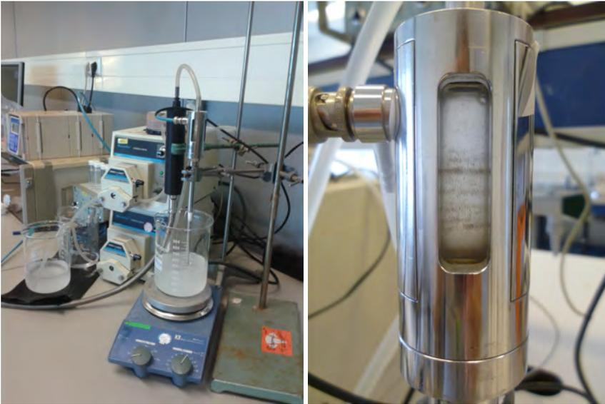
**Figure 8.2:** Experimental setup using a BioSep, two peristaltic pumps and an inline turbidity meter (left) and a zoomed in view of the BioSep resonator chamber (right).
