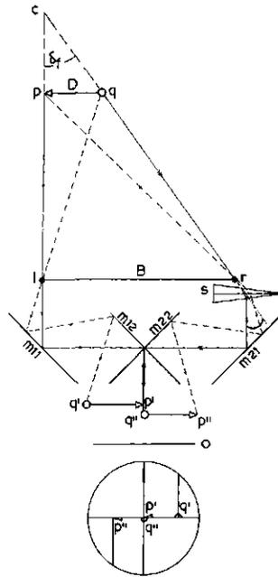
FIG. 2. False coincidence (schematically).
