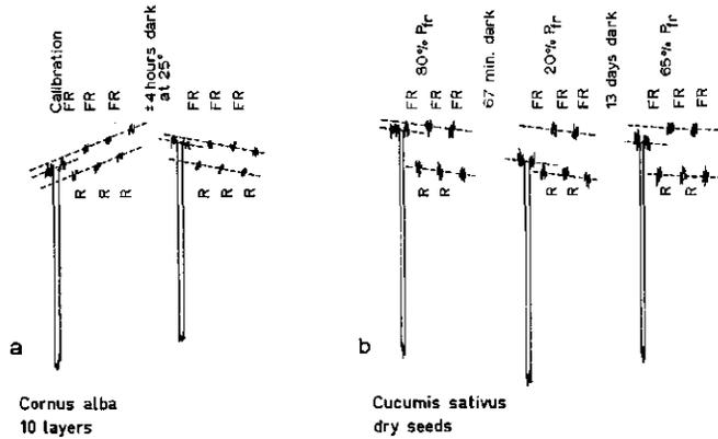
FIG. 14. Examples of phytochrome measurements, made with the dual purpose instrument, described under section 4. Two-wavelength mode, 730–806 nm. After writing a calibration mark, the traces were recorded during 30 sec each, with alternate exposures of the sample to actinic red (R) or far red (FR) light for 45 or 60 sec. Upward movement: increased absorption at 730 nm relative to 806 nm.
