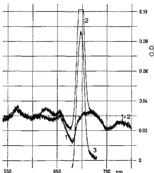
FIG. 13. Example of spectra, measured with the arrangement of fig. 11. Internode sections of dark grown pea, temperature  $-196^{\circ}$ .
