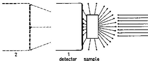
FIG. 1. In order to collect a maximum of scattered light, the distance between sample and photodetector should be as small as possible.
