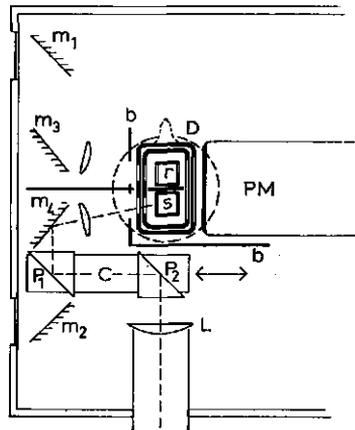
FIG. 11. Adaptation of the scattered transmission accessory of the Cary-14 spectrophotometer to irradiation of sample s inside a cryostat. D: cross section of dewar flask (see fig. 12). The 90° prisms P<sub>1</sub> and P<sub>2</sub> are mounted together on a carriage C. During spectrum recording, this carriage is slid out of the measuring beam. b: Baffles. r: reference sample, receiving no actinic irradiation.
