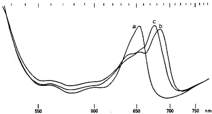
FIG. 9. Example of a recording, made with the instrument, shown in fig. 8, at low sensitivity. Leaves of dark grown maize, mounted between microscope slides. Reference sample was a suitable thickness of filter paper.
