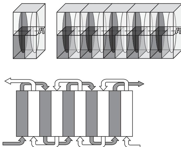
**Figure 1: Top: schematic of a single (left) and multi-unit (right) prototype of the Liquid gas liquid ammonia exchange system. Bottom: schematic top view of the manure flow (dark) and acid flow (light) through the apparatus.**
