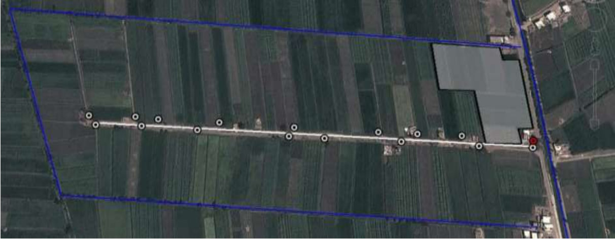
Figure 24 - Mesqa PS33; the non-PS area and un-used valve highlighted
