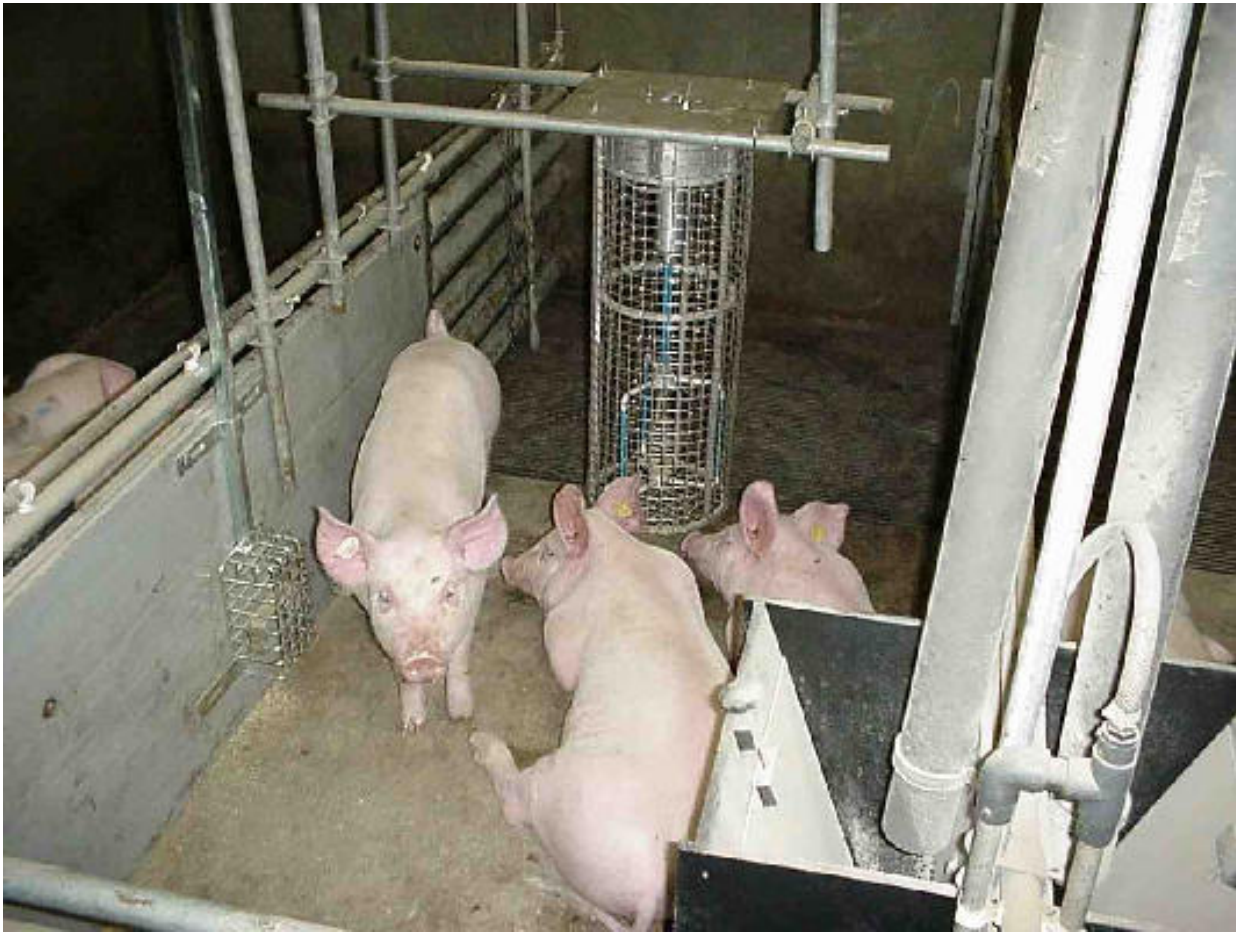
Figure 1. Air velocity anemometer in a wire cage in the middle of the pen.
