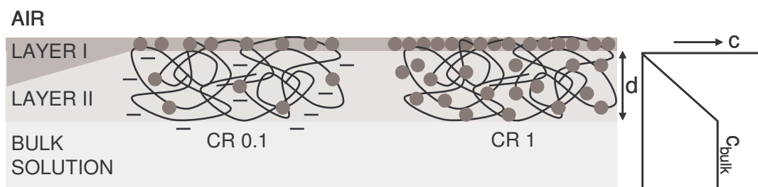
Figure 8.6: Schematic depiction of mixed adsorbed film consisting of two layers. Layer I has a thickness of \sim 4 nm and is in direct contact with air. Layer II is a thicker and more diffuse layer, the density of both layers depends on the protein/polysaccharide charge ratio (CR). For the estimation of an effective diffusion coefficient of protein through layer II (with a thickness 'd') the bulk protein concentration below layer II is indicated with ( c_{\text{bulk}} ). Layer I is considered as a 'perfect sink' for protein.
