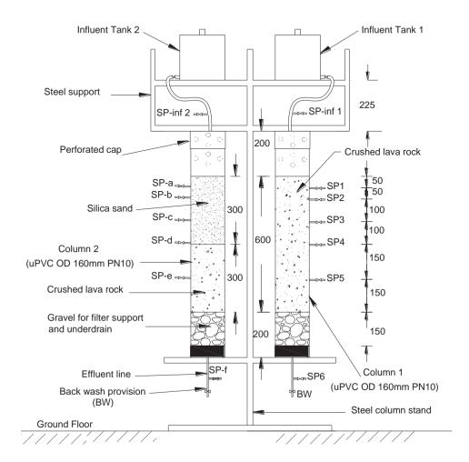
Figure 7.1: A cross-section of the column experimental set-up (SP refers to sampling point and all dimensions are in mm)
