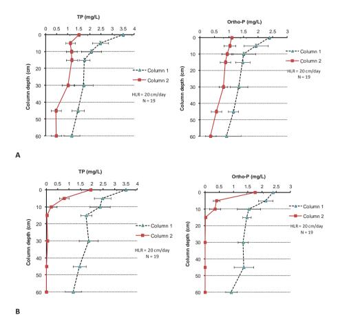
Figure 7.7: Total phosphorus (TP) and Ortho-P profiles after ripening period for A) column 1 (60 cm with lava rock) and column 2 (top 30 cm with sand and bottom 30 cm with lava rock) and B) column 1 (60 cm with lava rock) and column 2 (top 30 cm with granular activated carbon Norit GAC 830 W and bottom 30 cm with lava rock) operated at a hydraulic loading rate of 20 cm/day
