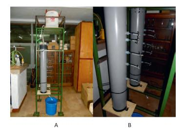
Figure 9.4: (A) Filter column set up and (B) location of sampling points on the two identical filter columns that were operated in parallel and in series
