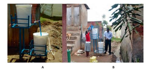
Figure 8.2: A crushed lava rock filter unit (A) implemented at a household near a tertiary drain to which the effluent is discharged (B) Grey water being poured into the filter unit, while samples are being collected
