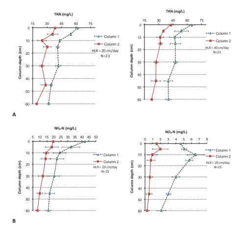
Figure 7.6: TKN, NH<sub>4</sub><sup>+</sup>-N and NO<sub>3</sub><sup>-</sup>-N profiles after ripening period for column 1 (60 cm with lava rock) and column 2 (top 30 cm with sand and bottom 30 cm with lava rock operated in series at constant hydraulic loading rates of 20 cm/day and 40 cm/day
