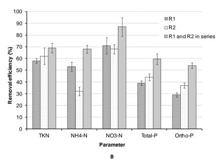
Figure 8.6: Removal efficiency of nutrients during grey water treatment by a two-step crushed lava rock filter after the ripening period at (A) a hydraulic loading rate (HLR) varying from 0.5 to 1.1 m.d<sup>-1</sup> and (B) a constant HLR of 0.39 m.d<sup>-1</sup>
