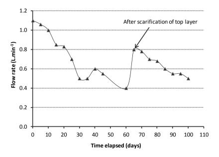
Figure 8.5: The flow rate at the outlet of reactor 2 after grey water charge during operation of the grey water filter after the ripening period (Hydraulic loading rate: 0.5 to 1.1 m.d<sup>-1</sup>)
