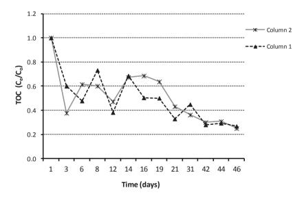
Figure 7.2: Evolution of COD and TOC removal during the filter columns' ripening period at a hydraulic loading rate of 20 cm/day. C<sub>e</sub> and C<sub>o</sub> refer to the TOC concentration in the column effluent and influent respectively
