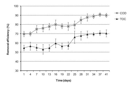
Figure 8.3: Evolution of the COD and TOC removal efficiency during the ripening period (Hydraulic loading rate: 0.5 to 1.1 m.d<sup>-1</sup>)
