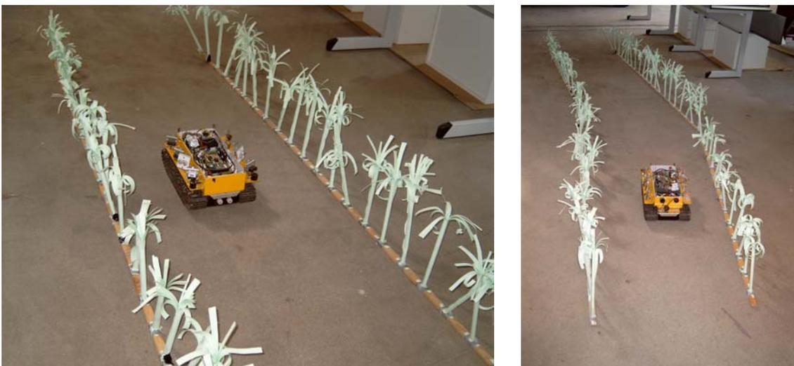
Figure 10. Cropscout between the artificial maize plants.
