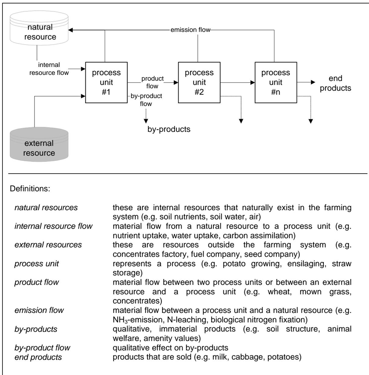
Fig. 3. Conceptual product flow model with its basic components
