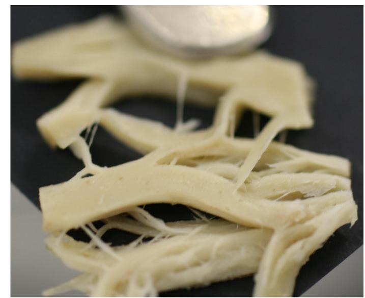
A pre-requisites to produce aligned hierarchical structure was simultaneous heating and shearing in a presence of gluten. The anisotropy of structures obtained was confirmed with a tensile test.
