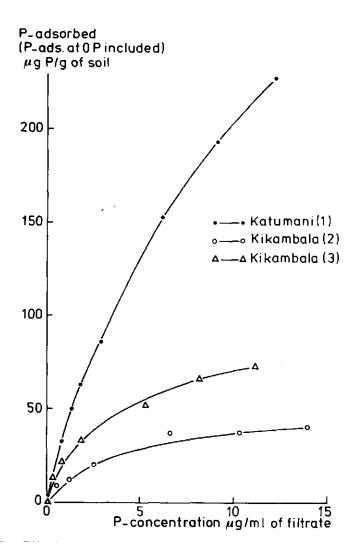
Figure 1. Phosphate adsorption curve for Katumani (1), Kikambala (2) and Kikambala (3) soil.
