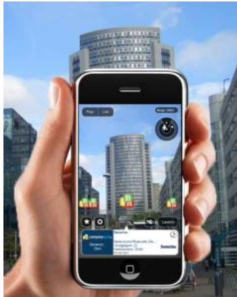
Figure 2 Accuracy problems. GPS on mobile phones do not provide enough accuracy in urban areas, which leads to miscalculations in GPS position and the misplacement of AR Features
