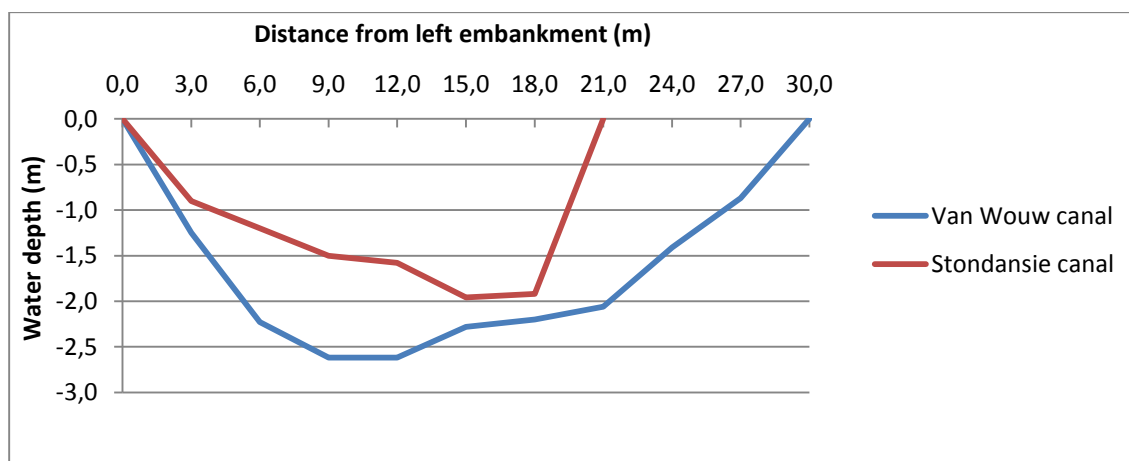
Figure 18: Cross-sectional depth profiles of Van Wouw canal and Stondansie canal near Nanni intake. 16-02-2012: Downstream water level= 1.99m+NSP
