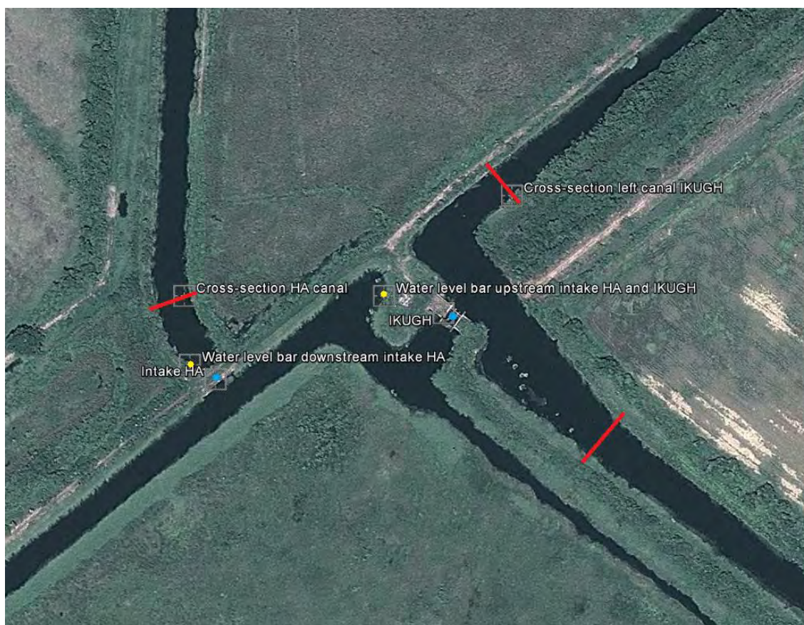
Figure 44: Google Earth picture with GPS-locations of intake HA and IKUGH (blue), the staff gauges (yellow) and the discharge measurement cross-sections (red). Derived at 21-03-2013
