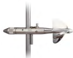
Figure 9: Velocity measurement instrument: Ott current meter. (Scottch, 2013)
