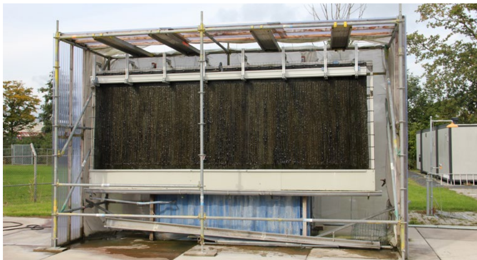
Figure 5.2 — The pilot-scale phototrophic biofilm reactor at the wastewater treatment plant in Leeuwarden.
