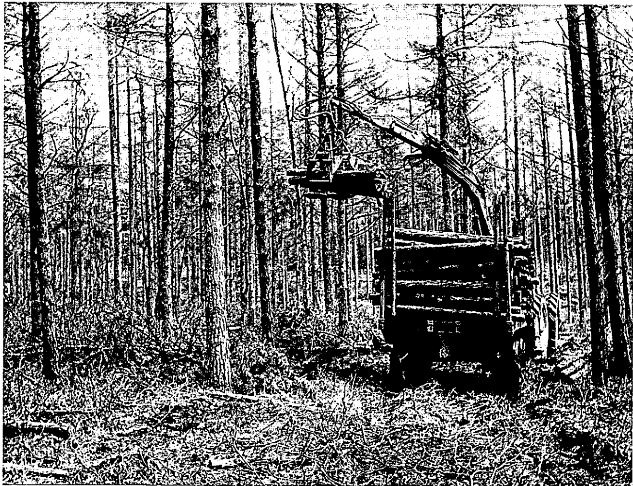
Foto 2. Sortimentenmethode; laden en lossen met hydraulische kraan. Photo 2. Shortwood method; loading and unloading by hydraulic crane.
