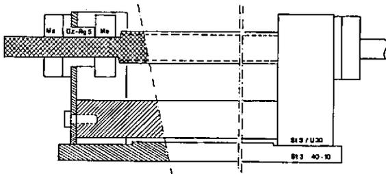
construction of spindle and support.
