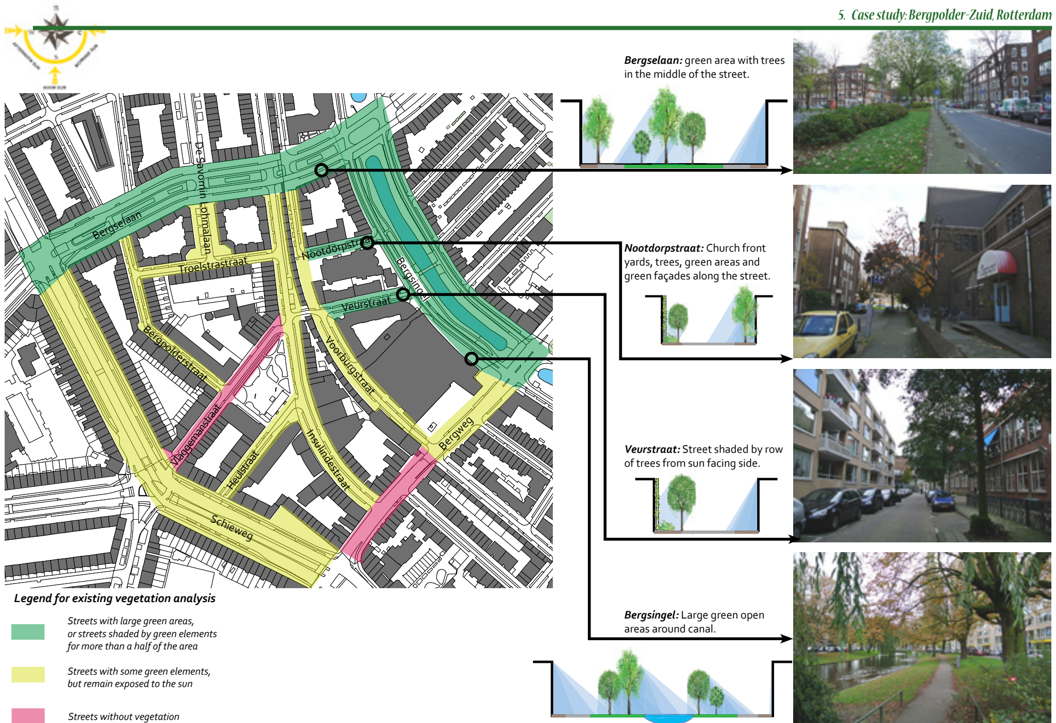
Figure: 5.20 Analysis of amount of green elements in the street and their shading impact
