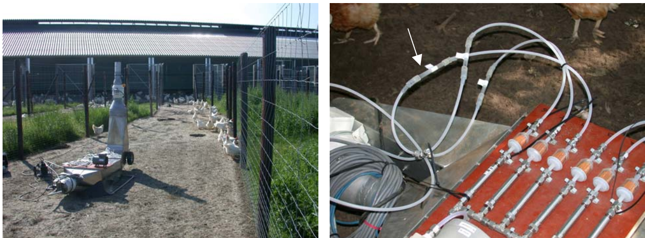
Figure 4. The ventilated chamber for measuring ammonia emission (left) and a detail of the denuder method equipment (the arrow indicates the location of the denuder).
