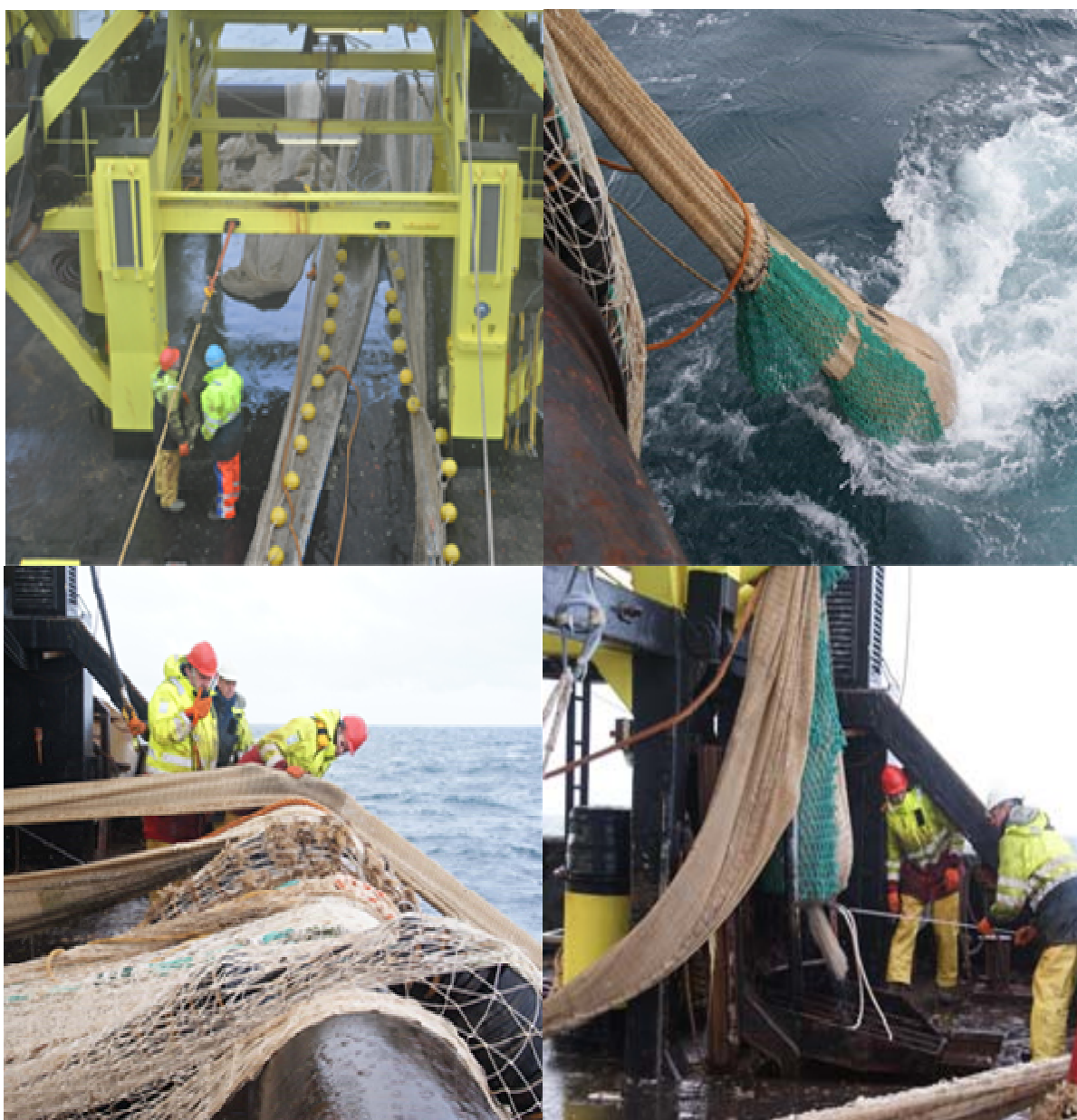
Photo 1 to 4: 1) the net hoisted on deck; 2) part hanging over board; 3) hoisting the codend, 4) emptying the codend.
