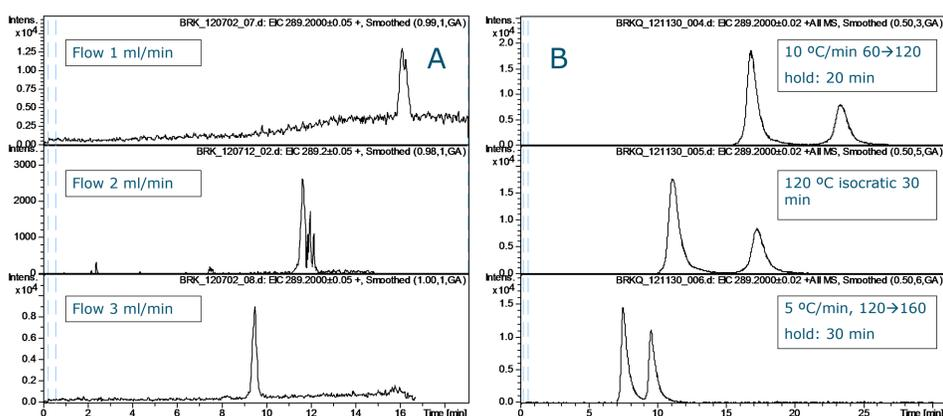
Figure 2. HTLC gradient optimization with  $\alpha/\beta$ -T on two Zirchrom columns (A) 100x4.6 mm, HT gradient: 60 $\rightarrow$ 120°C, 10 °C/min, hold 10 min (B) 100x2.1 mm, flow: 0.3 ml/min.
