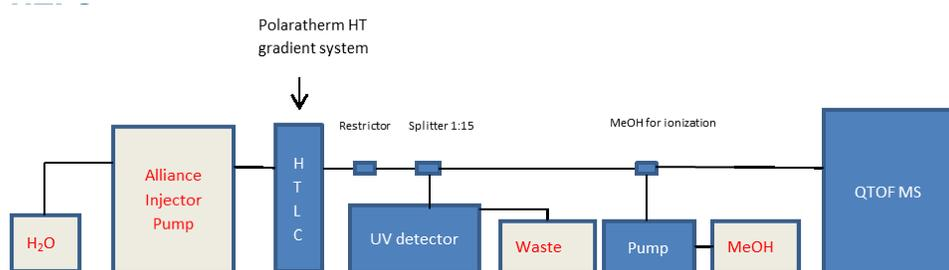
Figure 1. Schematic overview of HTLC-UV-QToF-MS set-up.
