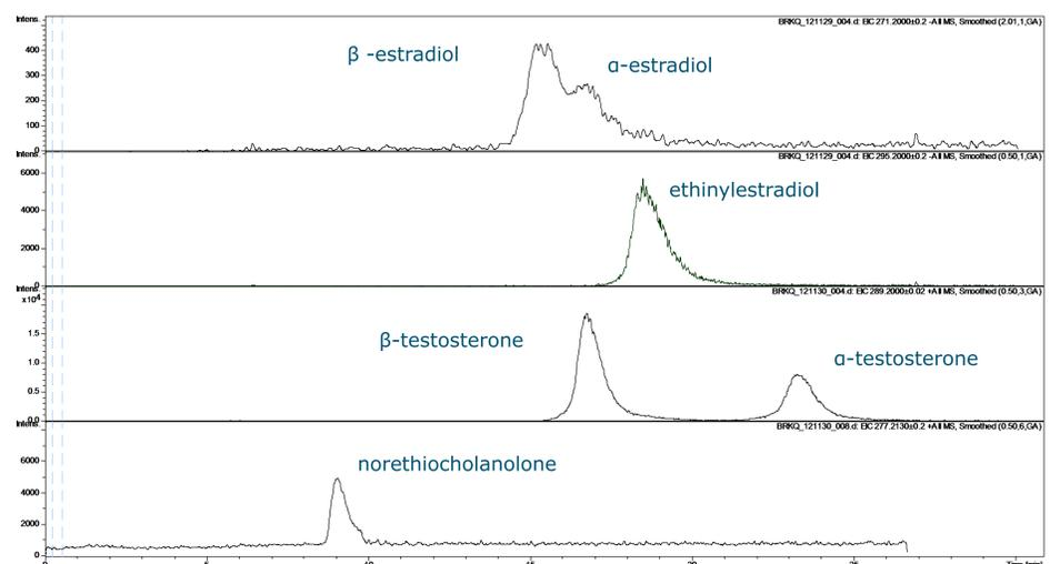
Figure 3. HTLC separation of hormones in bovine urine (Zirchrom 100x2.1 column, 0.3 ml/min).
