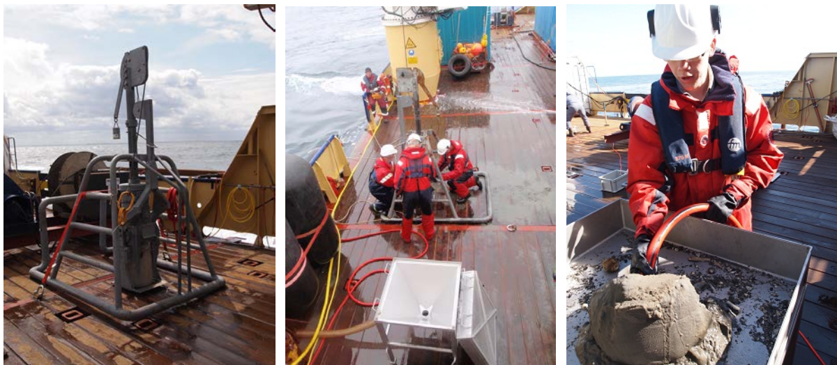
Figure 3: Box-corer on deck of the 'the Noortruck' (left), employment of box-corer (middle) and sieving of a sediment sample (right).
