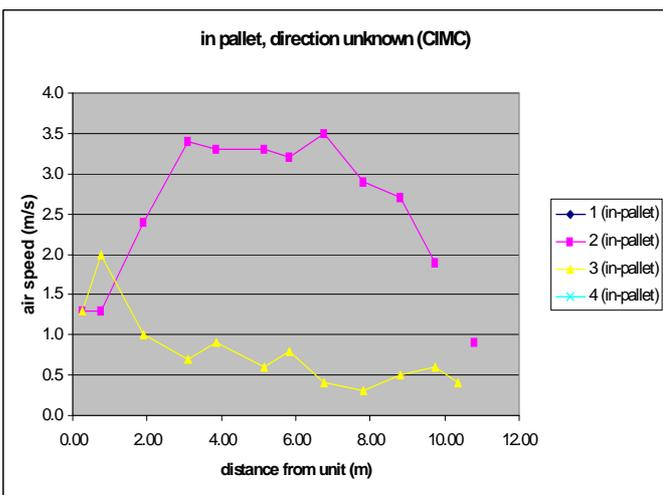
Fig. 15, air speeds in CIMC box with floor coverage.
