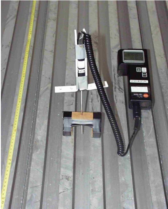
**Fig. 11, air speed measurement device used.**
