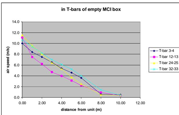
Fig. 12, air speeds in T-bars of SUDU 471502[2] while empty.
