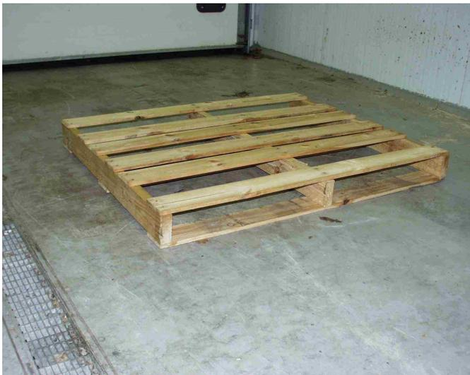
**Fig. 4, two-way pallets used.**
