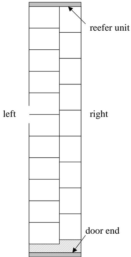
**Fig. 3, schematic top view of container stowage**
