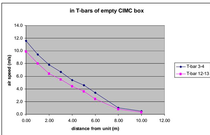
Fig. 13, air speeds in T-bars of SUDU 470597[6] while empty.
