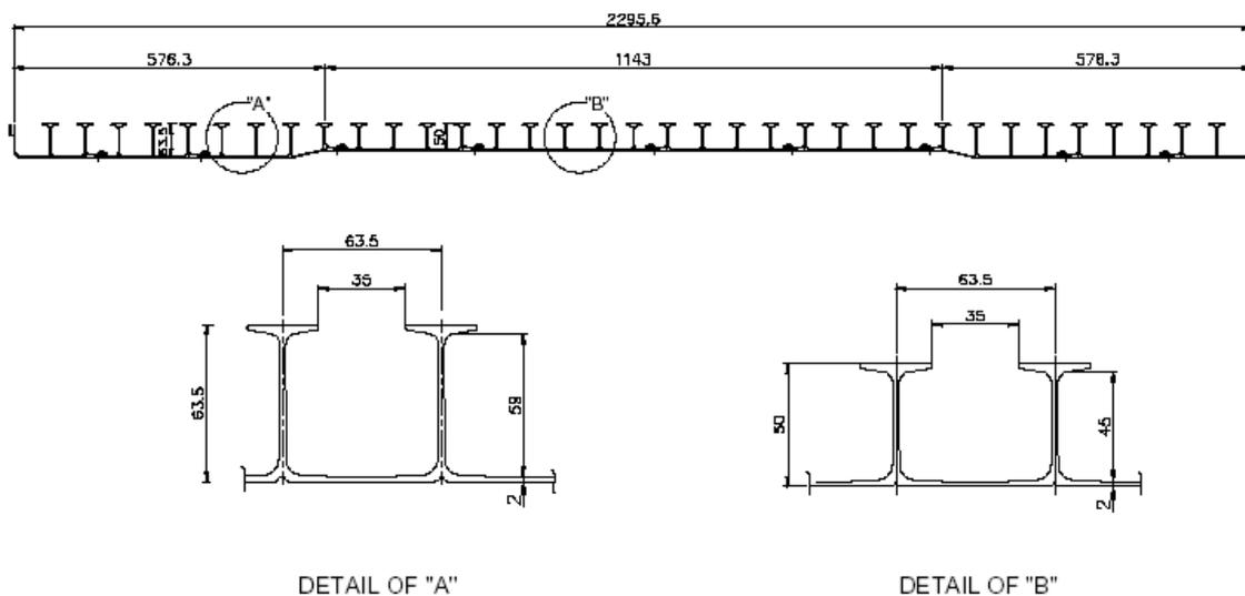
**Fig. 1, design drawing of T-bars in SUDU 471502[2].**
