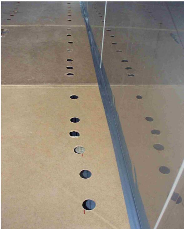
**Fig. 6, side chink closed with adhesive tape.**
