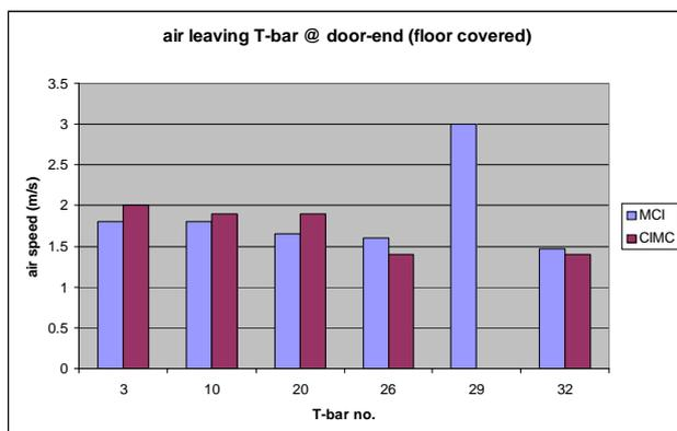
Fig. 16, air speeds leaving the T-bars at door-end
