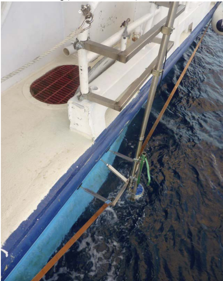
Figure 5. Acoustic Doppler Current Profiler (ADCP) attached to the research vessel.
