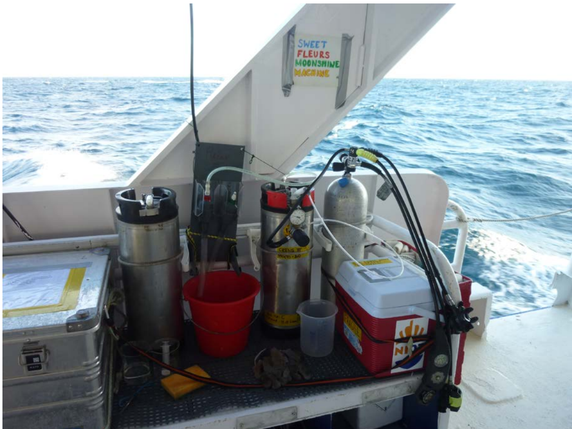
Figure 4. Experimental filtering set up with pressure vials and a dive tank. Filters were placed in the grey PVC filter holder in the middle.
