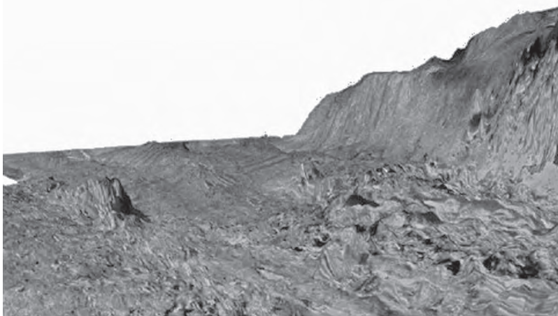
Kill van Kull, Newark Bay: Three dimensional sonar image with draped stratigraphy showing depositional zones in the channel bottom. The protruding topography at the base illustrates the bedrock diabase outcroppings that are scheduled for removal by drilling and blasting.
