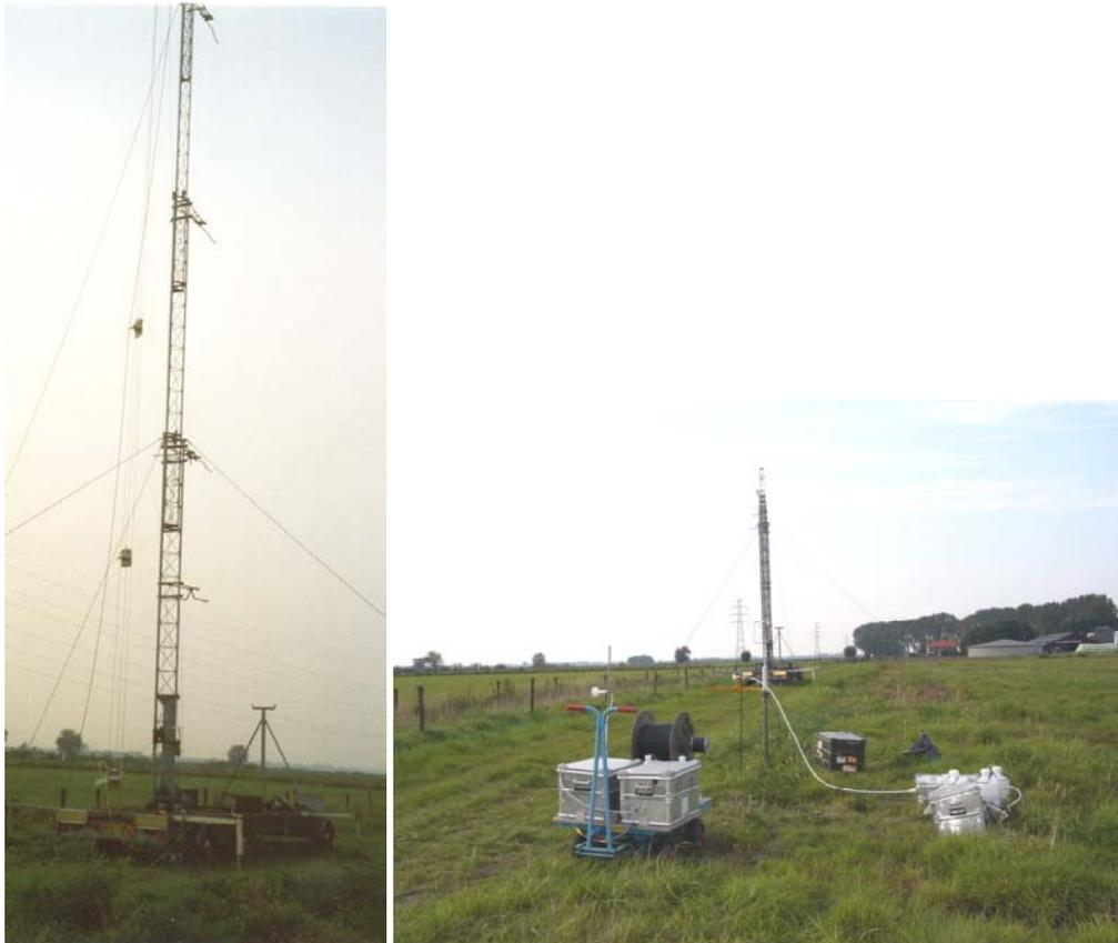
**Figure 3.7** Experimental set-up in Wageningen: a) denuders (4 heights) in a large (20 m) mast configuration; b) ECN fast sensor (left) and AMANDA system (right).
