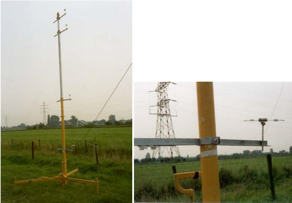
**Figure 3.8** Experimental set-up in Wageningen: ammonia passive flux samplers and Willems badges in a 5 m height-mast configuration.
