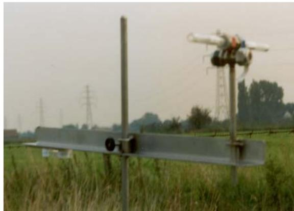
**Figure 3.9** Experimental set-up in Wageningen: ammonia passive flux samplers and Willems badges in a short-mast configuration.
