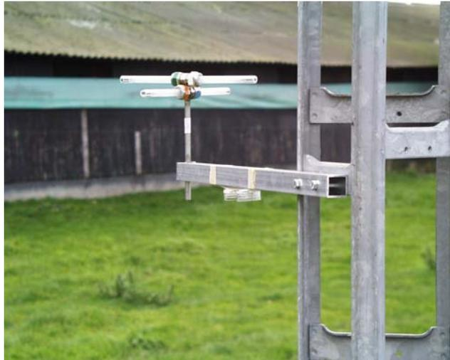
**Figure 3.15** Passive flux samplers in a cross design as used in Barneveld.
