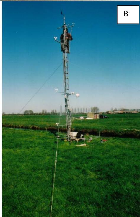
**Figure 3.2** Experimental set-up for ammonia concentration/flux measurements (Zegveld).
