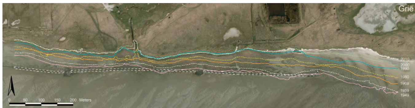
Figure 4. Aerial view of Grië, with the position of the marsh edge in 1949, 1959, 1969, 1980, 1990, 2000, and 2010 and the erosion protection works (dashed lines).
