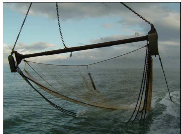
One of the 6m beam trawls used during the demersal survey. Attached to this beam is the 20 mm net. In the middle of the net, the CTD device is visible (Grift 2004).
