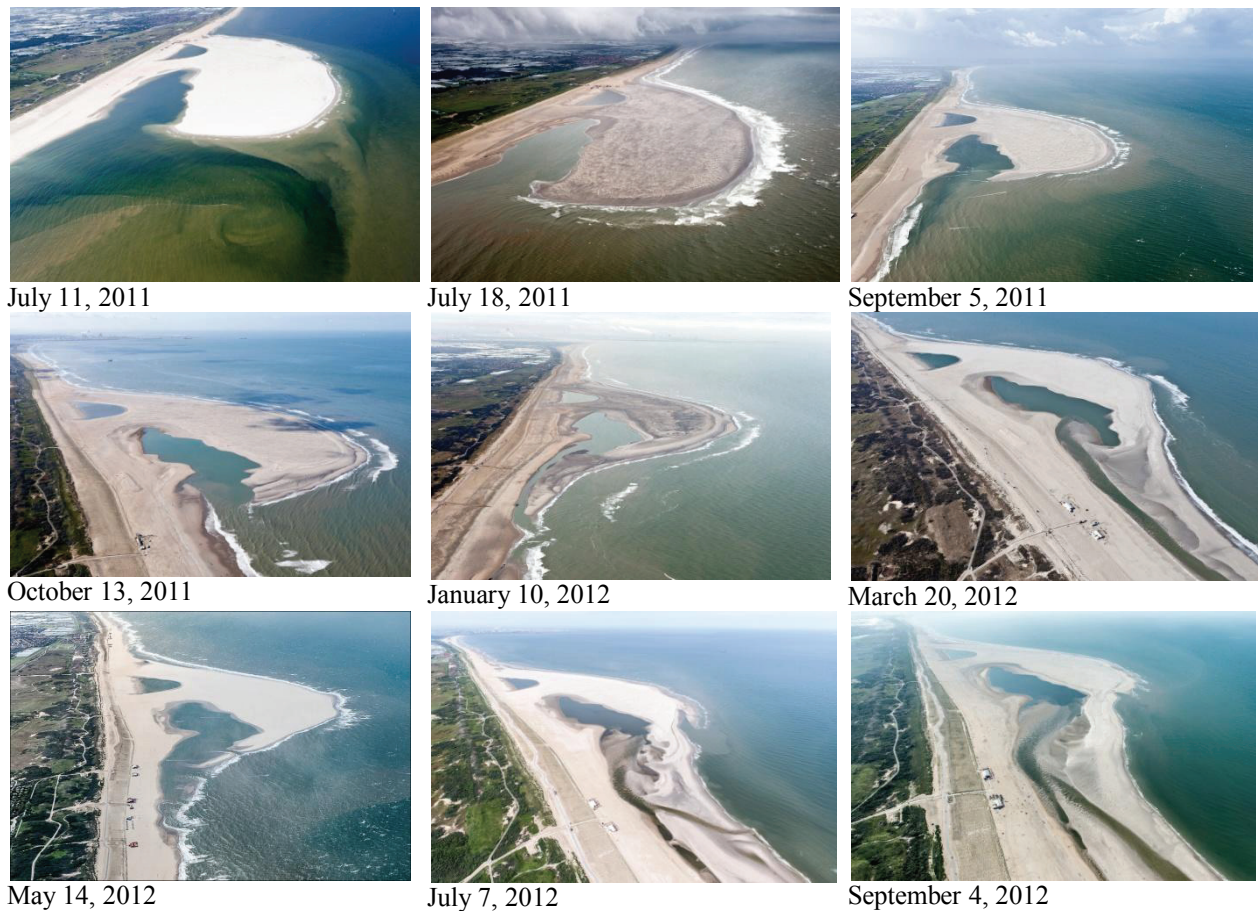
Figure 3. Morphological evolution of Sand Motor since completion early July 2011. Pictures courtesy of Rijkswaterstaat / Joop van Houdt
