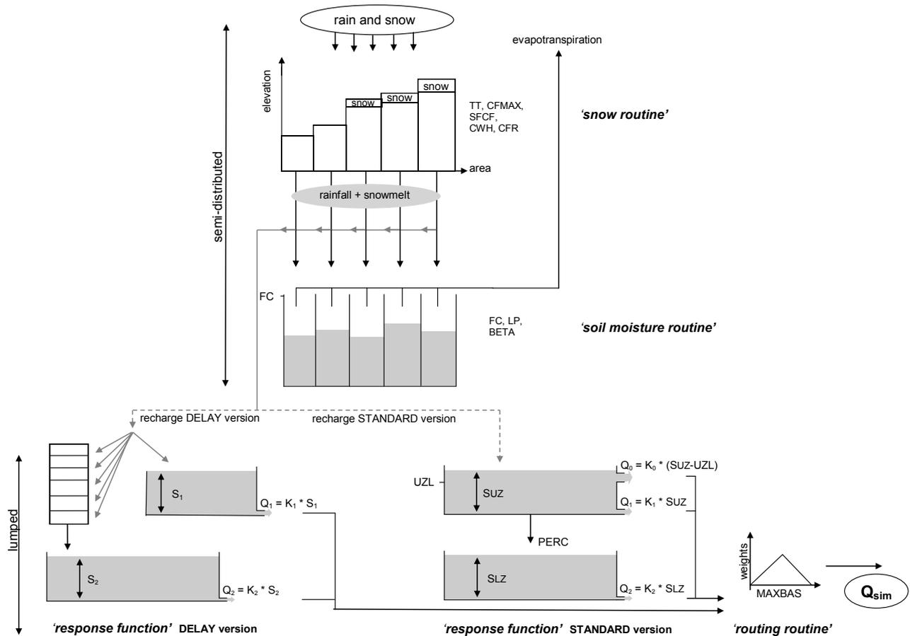
**Figure 2.5:** Structure of the HBV model with two versions for the response routine: on the right-hand side the STANDARD version, and on the left-hand side the DELAY version (adapted from Seibert, 2000 and Oosterwijk et al., 2009).
