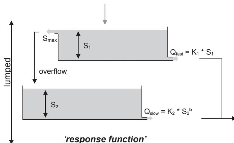
**Figure A.5:** Structure of the adapted HBV model, in which the response function of HBV is replaced by a linear reservoir overflowing into a non-linear reservoir (compare with Fig. 2.5).
