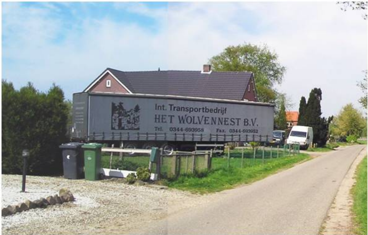
Fig 4. Re-use of an FFB in practice as a transport service. The capacity of the minor rural road seems to be slightly overloaded: the sandy verge on the right-hand side shows initial damage. (Picture: H. J. Sanders).
