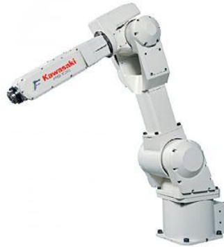
Figure 6. Kawasaki FS10E robot arm Source image: Kawasaki Robotics Inc. Product Specification.
