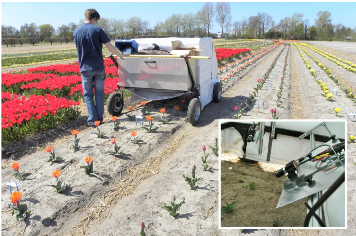
FIGURE 1: The imaging platform in the field. The inset shows the interior, with the two color cameras.
