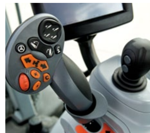
▲ De forced-based handle bedient vele taken.
