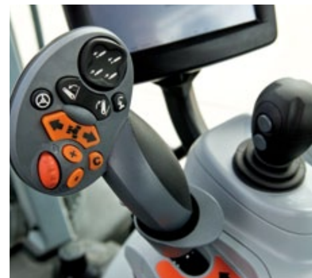
▲ De forced-based handle bedient vele taken.
